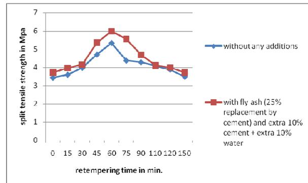
**Figure 2:** showing variation of split tensile strength.
