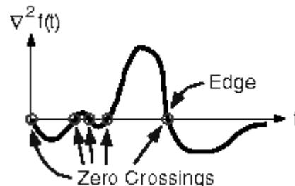
Fig.2.4(c): Identification of Zero Crossing
