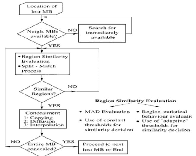
Fig. 1. Flowchart of the FEC algorithm.
