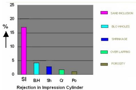
Fig.2 Percentage of rejection in impression cylinders
