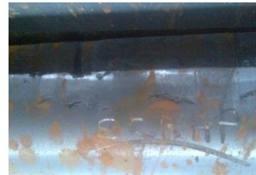
Fig.5 Diagram of sand inclusion
