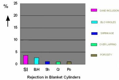
Fig.4 Percentage of rejection in blanket cylinders
