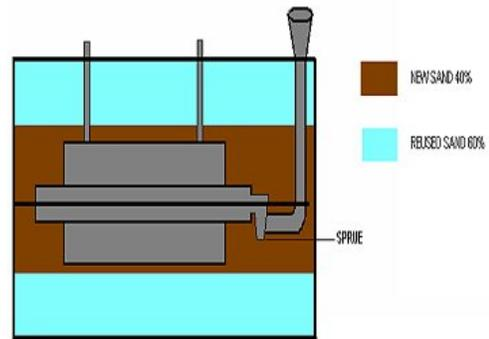
Fig. 15 Diagram of suggested system
