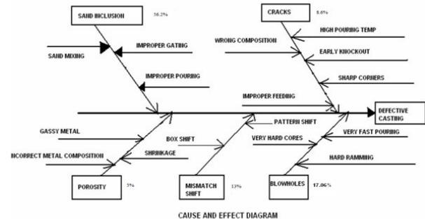
Fig.10 Cause and effect diagram of casting defects
