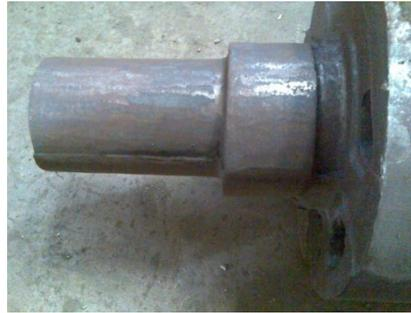
Fig.8 Diagram of mismatch shift.
