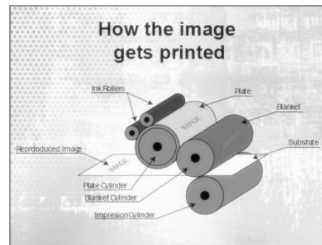
Fig 1 Schematic diagram of offset printing press
