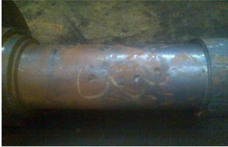
Fig.6 Diagram of blowholes
