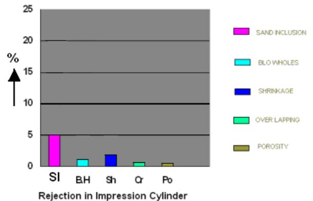
Fig.16 Represents percentage of rejection after the suggested method
